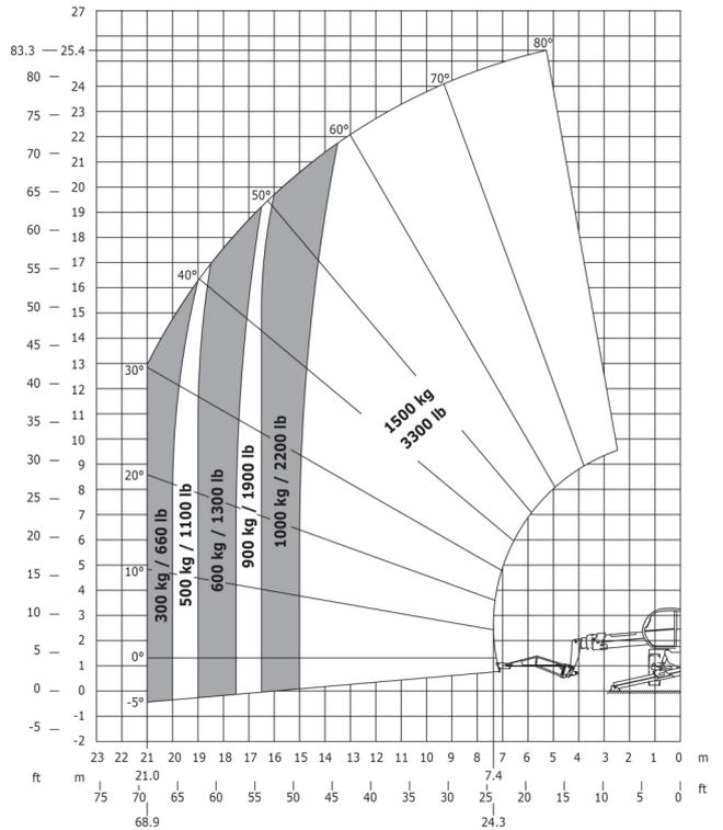
Rotation on lowered stabilisers with 365 kg platform
