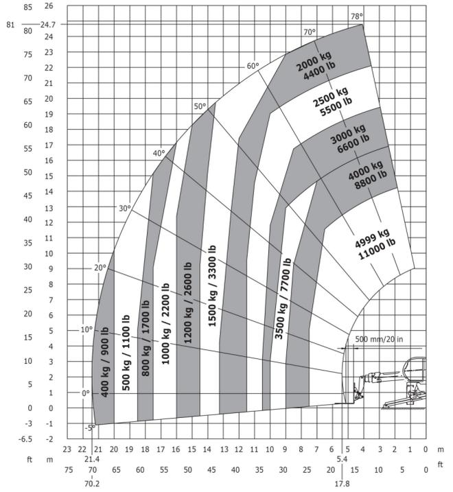
Rotation on lowered stabilisers with winch 5000 kg
